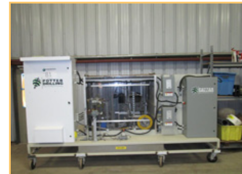
CUSTOM CHEMICAL MIXING AND PUMPING SKID
