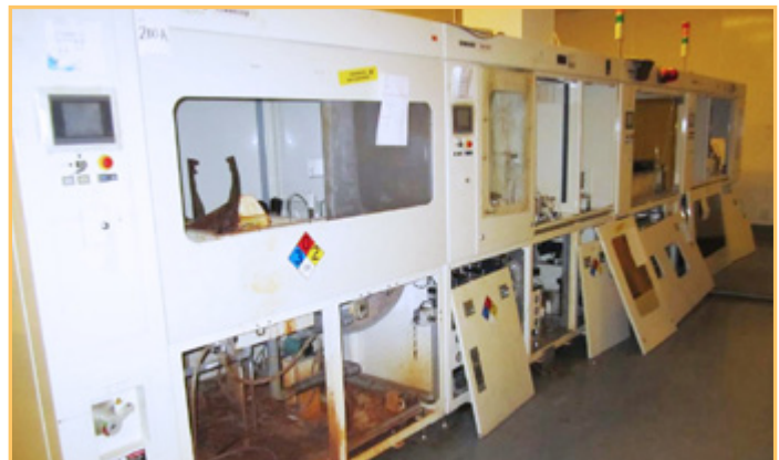
SONY CD GLASS MASTERING LINE, UPGRADED WITH SOLID STATE LASER AND ECLIPSE 8.0 CODER
