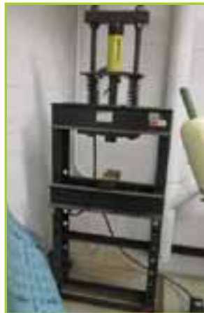
DAYTON 32916A 25 TON HYDRAULIC PRESS, TYPE H-FRAME
