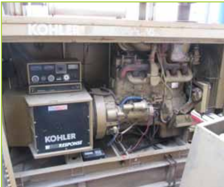
WHITE/KOHLER WHITE 100KW DIESEL GENERATOR , HOURS 1051, S/N 4019462, 150 GAL TANK, WITH 300 GAL DAY TANK, KOHLER GENSET MODEL 100R0Z71
