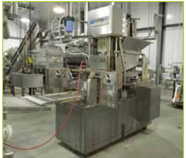
(2) FORMAX PATTY FORMERS MODEL PFM19, S/N 306 AND MODEL F19 S/N 428, WITH TENDERFORM SYSTEM, CUBERS, AND DUMPERS
