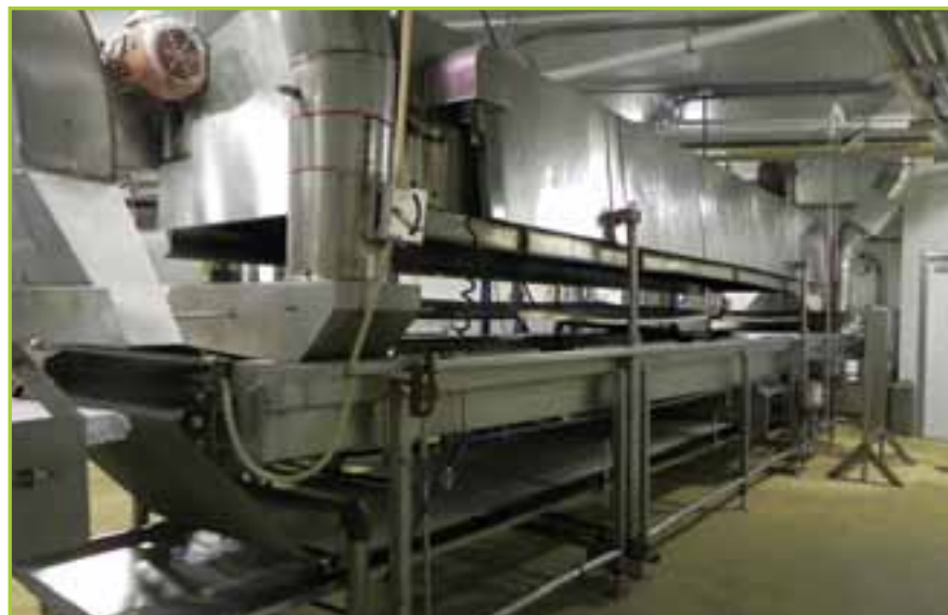
STEIN DEEP FRYER, MODEL: HPF114405G, SN: 462, W/ HYDRAULIC SYSTEM, FILTERS, AND S/S TANK
