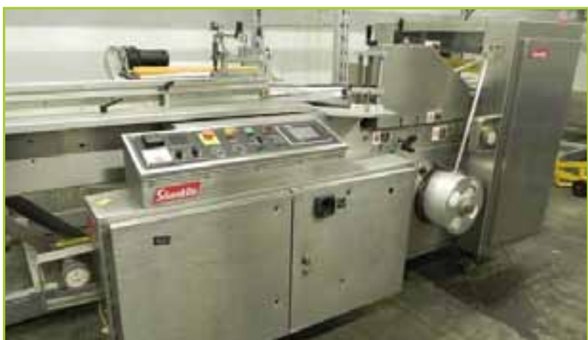
SHANKLIN FLOW WRAPPER, MODEL: F-555, W/ PLC CONTROLS, SCRAP WINDER, AND DAMARK HEAT TUNNEL
