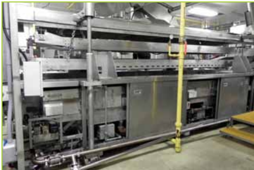
TETRA LAVAL FOOD KOPPENS S/S HLT OVEN, MODEL: HLT 8000/1000, SN: HLT 8000/1000-153, W/ ALLEN BRADLEY CONTROLS, 40 FT. LONG X 40" WIDE
